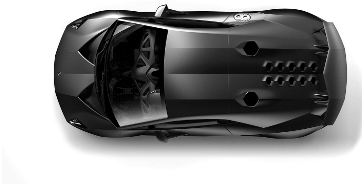
Figure 1.1 In October 2010 Lamborghini introduced the Sesto Elemento concept car, a technology demonstrator with 80% of its total weight of 999kg made of carbon CFRP. Besides the monocoque, several structural parts were made of carbon CFRP: the transmission shaft, the front subframe, the crash boxes, and parts of the suspension. Photo: Automobili Lamborghini S.p.A. (with permission).
